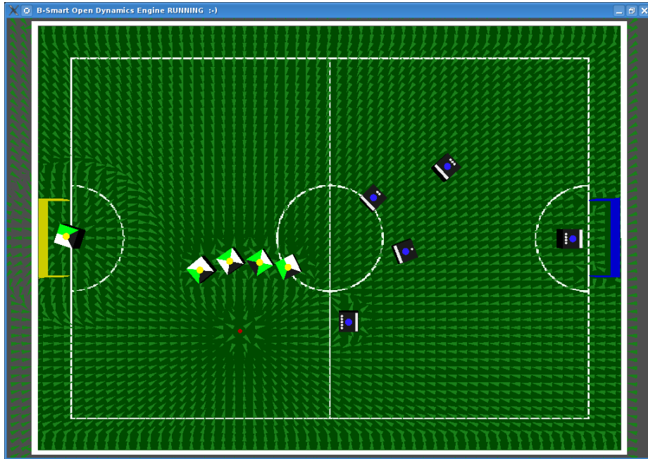
Fig. 5. A potential field for moving during the STOP state.
